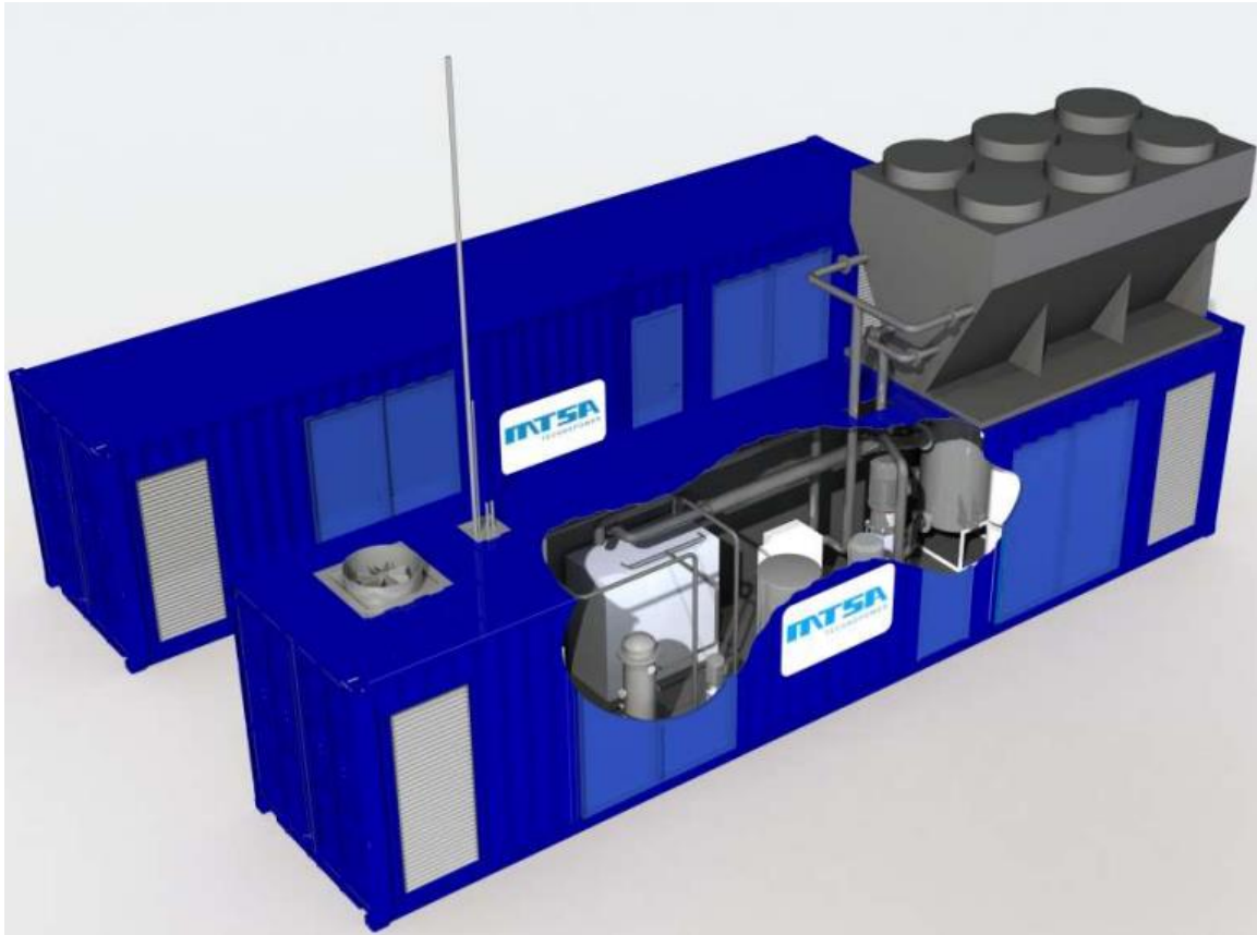
Figure 4.10: Schematic representation of two 1 MW elektrolysers including cooling tower (grey top area)
